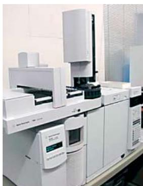
**New toys at NWU, Potchefstroom: Agilent 5975C GCMS, equipped with a 7890A GC and 7693 Autosampler.**
